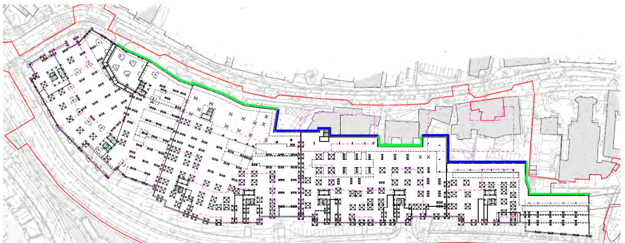
Figure 5-10: Foundation Structure Layout
